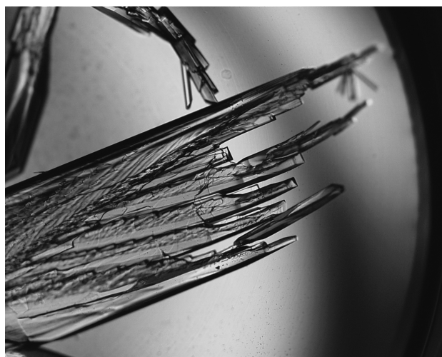
Fig. 2. Alpha-amylase crystal grown in terrestrial gravity by the vapour-diffusion method
